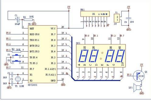
Note: there is direction for PR1 Resistors-Pack; there is one side of the word in the direction of the IC. Pay attention!!!
