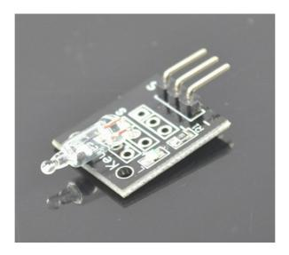
Mercury switch module and a digital interface, built-in 13 LED build a simple circuit to produce tilt warning lamp
