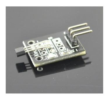
Hall magnetic sensor module and a digital interface, built-in 13 LED build a simple circuit to produce a magnetic flasher.
