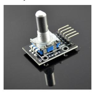
By rotating the rotary encoder can be counted in the positive direction and the reverse direction during rotation of the output pulse frequency, unlike rotary potentiometer counter, which
