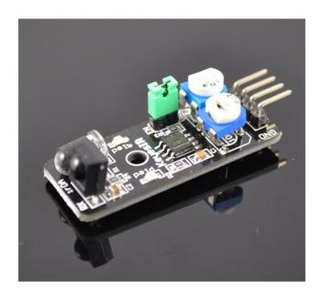
Infrared obstacle avoidance sensor is designed for the design of a wheeled robot obstacle avoidance sensor distance adjustable. This ambient light sensor
