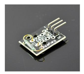
Reed module and the interface comes with digital 13 LED build a simple circuit to produce a Reed warning lamp
