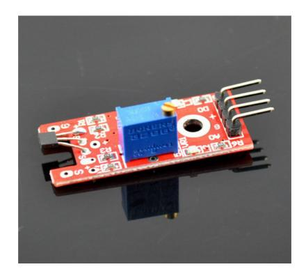
Linear Hall magnetic module and a digital interface, built-in 13 LED build a simple circuit to produce a magnetic field warning lamp
