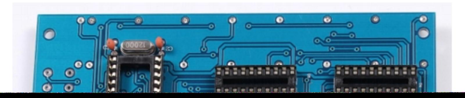
Step 6: Weld other components except LED and install ICs.
